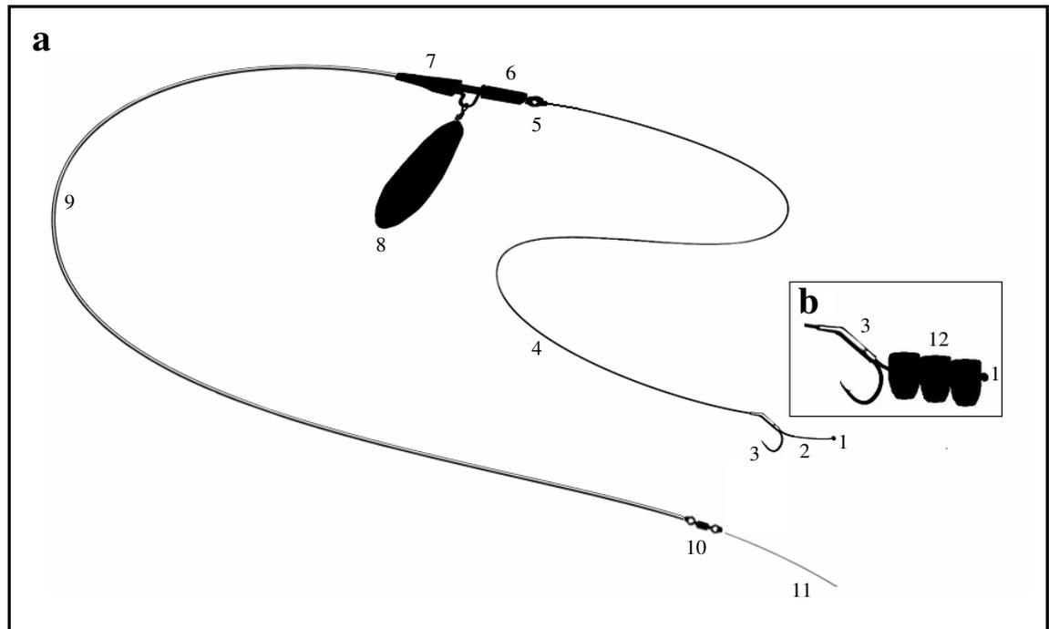
**Figure 3:** Illustrations of the angling rig used in this study (plot a) and the hair baited with corn (plot b): 1: boilie stopper, 2: hair, 3: hook, 4: leader, 5: swivel, 6: plastic clip, 7: rubber tube, 8: lead sinker, 9: braided line with a lead core, 10: swivel, 11: braided main line, 12: corn (modified from Rapp *et al.* 2008).
